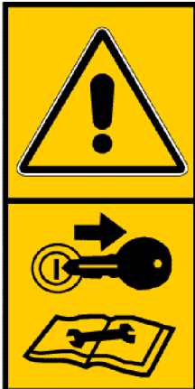
Shut off the engine and remove the key before performing maintenance or repair work on the machine.
