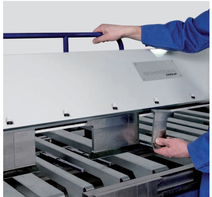
The MAKV S with its patented quick eccentric clamping device enables an easy and fast change of clamping beam tools.
