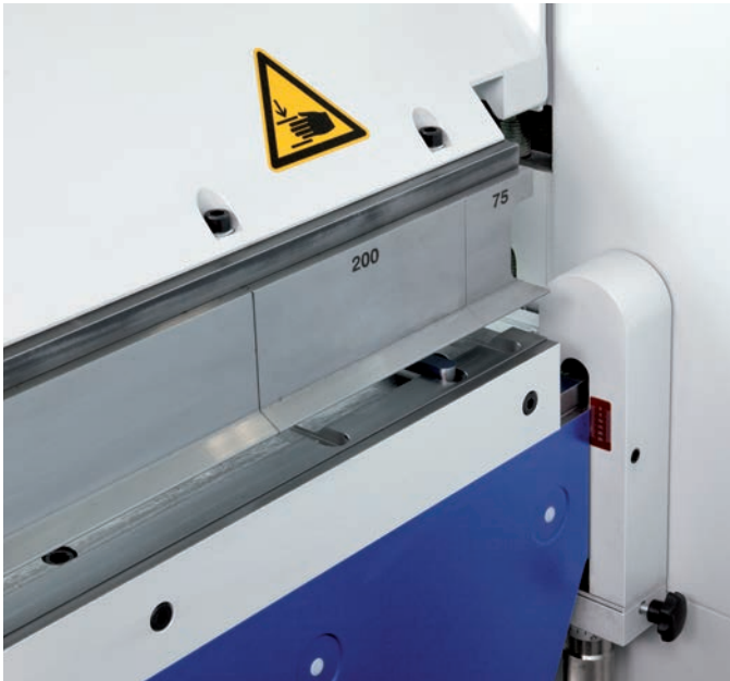
The MAKV with a popular tool option: the segmented goat's foot tool.
