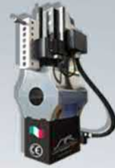
• MFH Motorized Facing Head:
