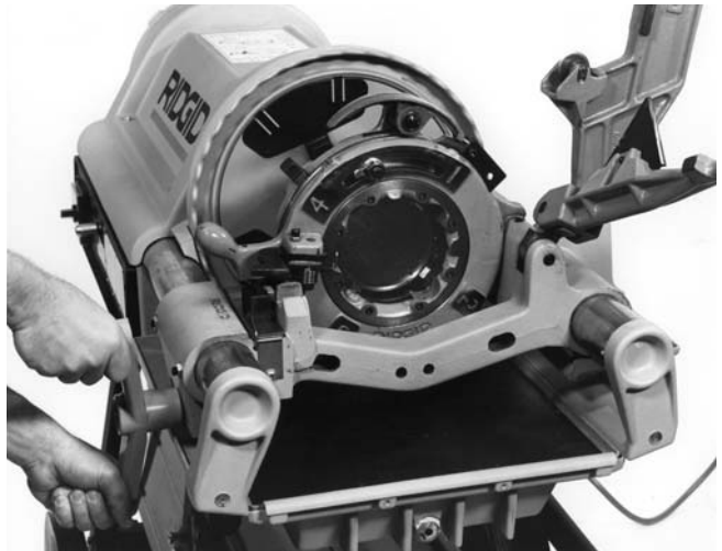
Figure 16 – Threading NPSM/BSPP Threads with No. 714 or 914 Die Heads
